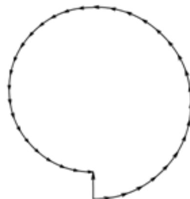
$$\vec{A}_{\text{рез}} = \vec{A}_1 + \vec{A}_2; A_{\text{рез}} \approx 0; I \approx 0$$
