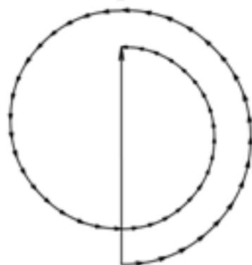
$$\vec{A}_{\text{рез}} = \vec{A}_1 + \vec{A}_2 + \vec{A}_3; A_{\text{рез}} \approx A_1; I \approx 4I_0$$
