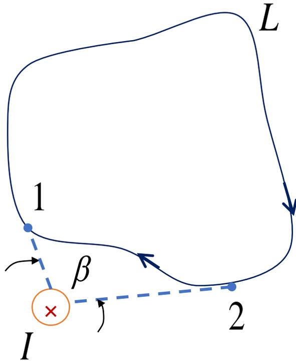
$$\oint_L \vec{B} d\vec{l} = \frac{\mu_0 I}{2\pi} \oint_L d\alpha = \frac{\mu_0 I}{2\pi} \left( \int_1^2 d\alpha + \int_2^1 d\alpha \right) =$$
